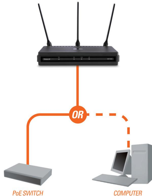
Connect one end of an Ethernet cable (included with your access point) to the LAN port on the DAP-2553 and the other end of the Ethernet cable to either your computer or to your PoE switch. The AP can be powered on by a PoE switch or by the power adapter shipped with the AP.
