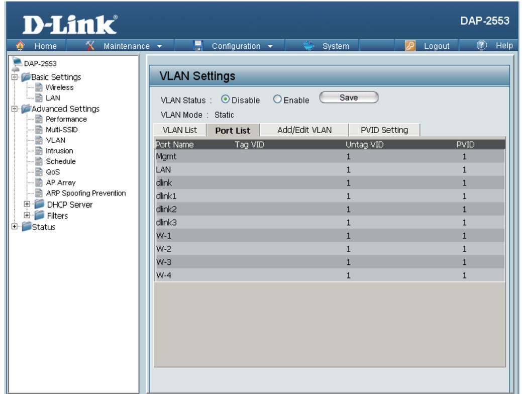
The screenshot shows the D-Link DAP-2553 web interface. The left sidebar contains a navigation tree with categories like Basic Settings, Advanced Settings, and Status. The main content area is titled 'VLAN Settings' and includes a 'VLAN Status' section with radio buttons for 'Disable' (selected) and 'Enable', and a 'Save' button. Below this is the 'VLAN Mode' set to 'Static'. The 'Port List' tab is active, showing a table with the following data:
